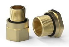
EXAMPLE PART NUMBERING: AR1BF/NP/M20/M25 Thread converting Adaptor/Reducer No IP O-ring(0) - Nitrile (1) - Silicone (3) Brass (B) - Stainless Steel (S) - Aluminium (A) Multiple Certification Locknut & Nylon (K), Fibre (V) or PTFE (H) IP Washer Including Earth Tag s Including Serrated Washer Quantity per kit Nickel Plated NP M20 Male Entry Thread Female Entry Thread
